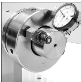
5 | Set the dial gage over the hydraulic nut
